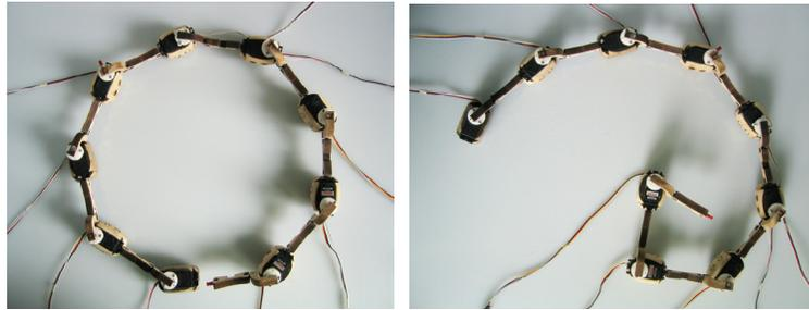
A Queen does not need to be mechanically attached to the creation it is programming, so it can also be used as a remote controller. Remote programming with a Queen gives a child synchronous input and output feedback during programming, allowing the child to observe their creation's motion while they are composing it.
