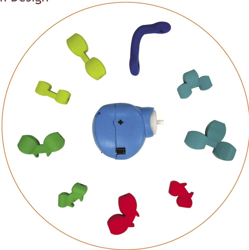
The Topobo system is comprised of ten primitives that are connected with Lego Technics® connectors. Nine of these primitives are called "Passive" because they form static connections. One motorized "Active" forms dynamic connections which allows the system to reproduce manipulations to a structure.
