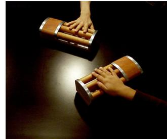
Super Cilia Skin is inspired by wind swept grass and explores how motion in an array of hair like actuators can be used as a textural communication device.
