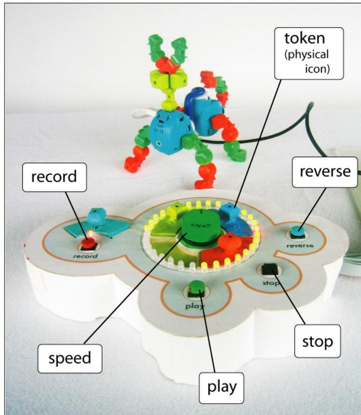
To playback this motion, the user will move the wooden token to one of four slots in a donut-shaped “playback arena,” and press Remix’s “play” button. Green lights beside the token signify that it is mapped to a recording, and a red marquee light advances as the recording plays (fig. 4). The user may turn a green knob on Remix to change the rate of playback, or push a button to change the direction of playback. She can sequence up to four distinct recordings to loop in the playback arena.
