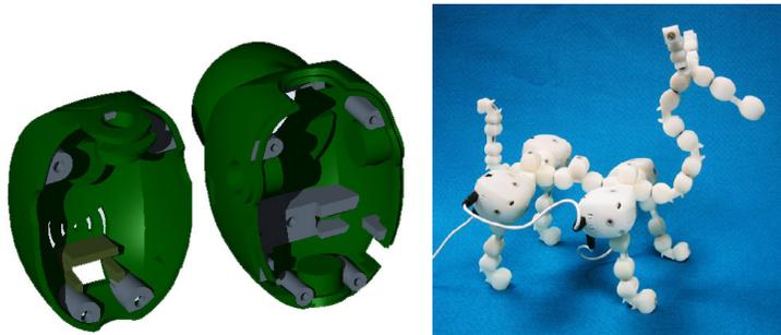
Second generation parts were modeled with 3D CAD software and 3D printed in ABS plastic. This allowed us to house the electronics and motor in a single case. Parts were later mass produced based on this design.
