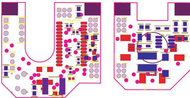
Topobo is based on modular robotics technology. Electronics inside every Active handle local memory and processing and power distribution. A custom peer to peer serial network allows Actives to communicate with each other through small, white cables.
