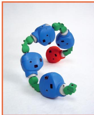
actives connected with tetrahedral passives create a spring-like helix when controlled by a queen.
