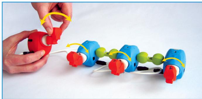
Special orange actives called Queens can control many other Actives. In both record and playback, all motions made to a queen are mimicked by the other actives connected to the Queen.
