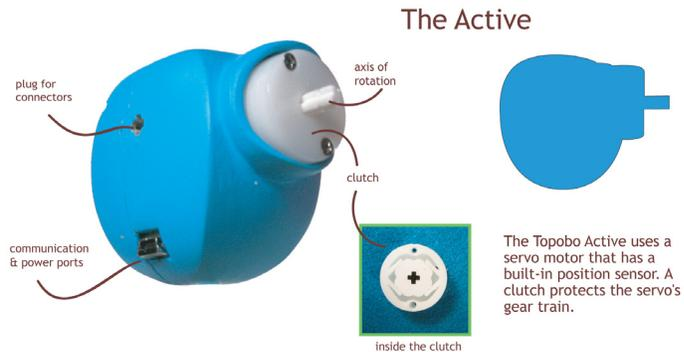
The Topobo Active uses a servo motor that has a built-in position sensor. A clutch protects the servo's gear train.
