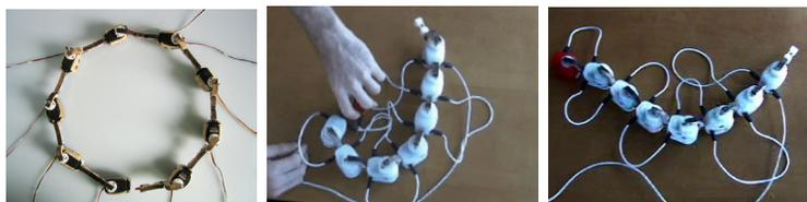
With the same motion, children can experiment with how Backpacks can affect a global behavior. A Queen leads to a circle. Adding a Bigger/Smaller Backpack creates a spiral. Using a time delay backpack forms a wave.
