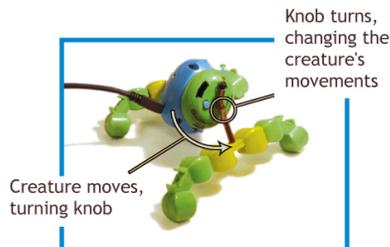
its knob used as a joint, a backpack introduces the idea of feedback
