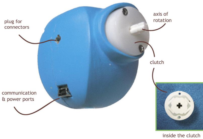
The Topobo Active uses a servo motor that has a built-in position sensor. A clutch protects the servo's gear train.
