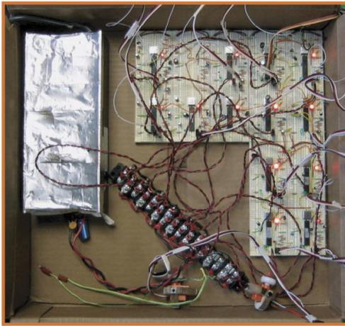
In order to avoid the “spaghetti” of wires we had with our prototypes, we needed to design a power distribution scheme to power all of the parts in a creation through one daisy-chained set of cables
