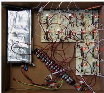
We built two prototypes to test the system design and concept. The cricket prototype tested the Queen and the breadboarded version tested a scalable, distributed electronic architecture.
